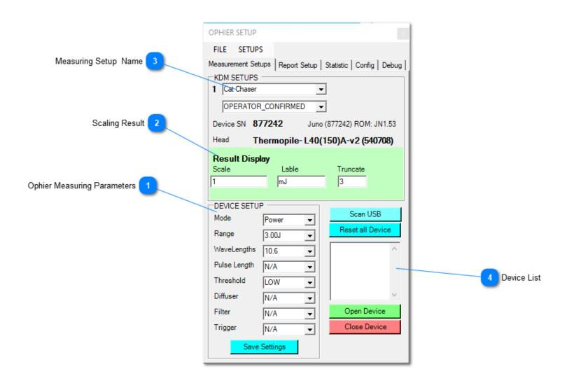
**Ophier Measuring Parameters** DEVICE SETUP Mode Power • Range 3.00J WaveLengths 10.6 Pulse Length N/A • Threshold LOW • Diffuser N/A Filter N/A • Trigger N/A •
