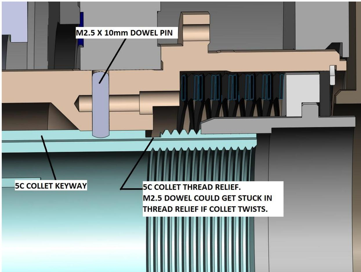
The 5C collet needs to be guided out of the DDR with one hand, while the other hand turns the back handle. This requires the “Toggle Mode” to be on, so that the spring is compressed and the spindle will not turn.
