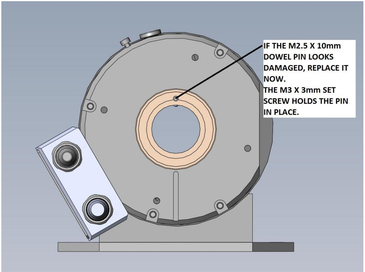
If replacing the M2.5 dowel pin, do not re-use the M3x3mm set screw (install new one). Make sure when installing a new M2.5 dowel pin to insert the tapered end first into the spindle. DO NOT force the pin into the hole, it should go in easily. If forced into the hole, it may not be removable ever again.
