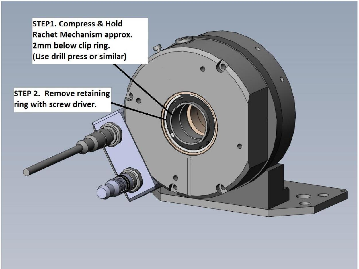
3. Remove Ratchet Mechanism and pull out DDR Spring.
