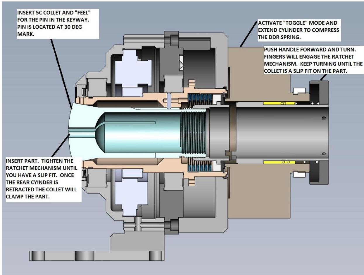
Activate the "Toggle" mode on the machine (Press and hold the collet button and then the reset button, and then let go of both). Press the collet button and watch the rear knurled black handle of the DDR move inwards towards the back of the cylinder (3mm Max, if more, adjust stop ring) and stay compressed. This will hold the spindle in place while tightening the 5C collet.
