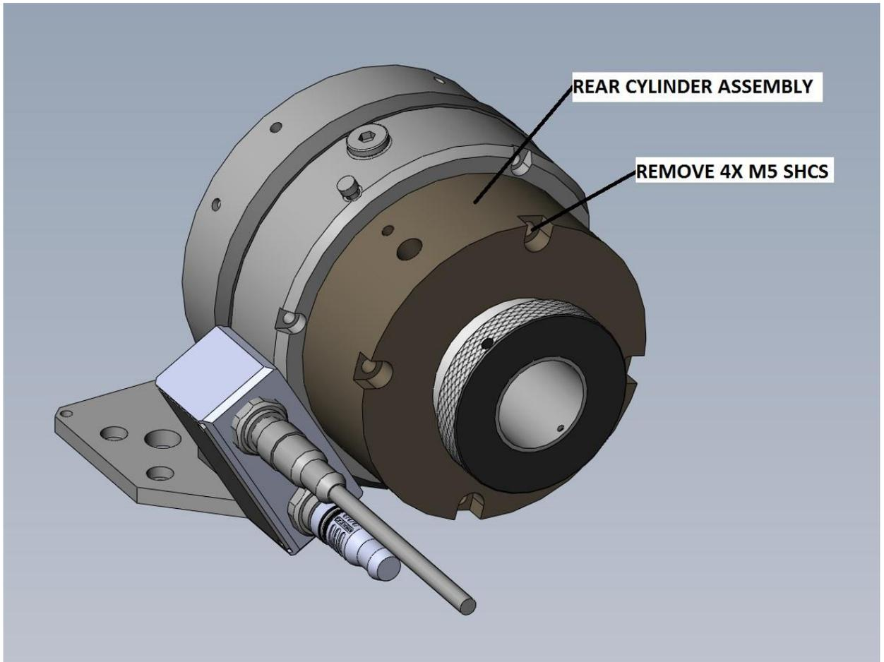
2. Compress 300lb DDR spring with Mill or Press approximately 2mm.
