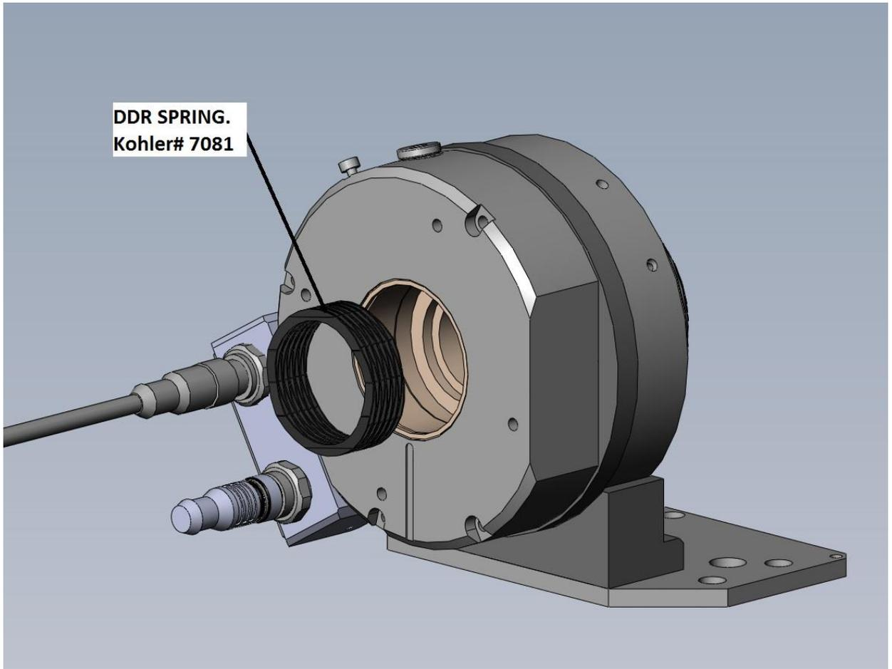
4. If the 5C locating dowel pin (M2.5 x 10mm) looks damaged replace it now. If not, Insert new DDR spring, and reverse the procedure.
