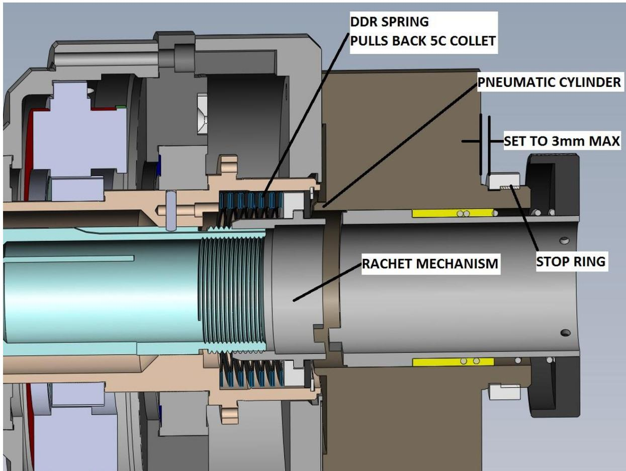
A broken spring can occur if the stop ring is set to more than 3mm. Most occurrences occur because the white delrin stop ring breaks, which allows the pneumatic cylinder to travel more than 3mm. This over traveling causes the spring to fatigue and break. Kohler Design has an aluminum replacement now available (Kohler# 100.5219B).
